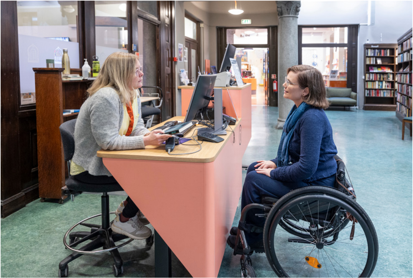
EYE LEVEL: Height-adjustable desks ensure access for and eye contact with all users: high and low, sitting and standing.
